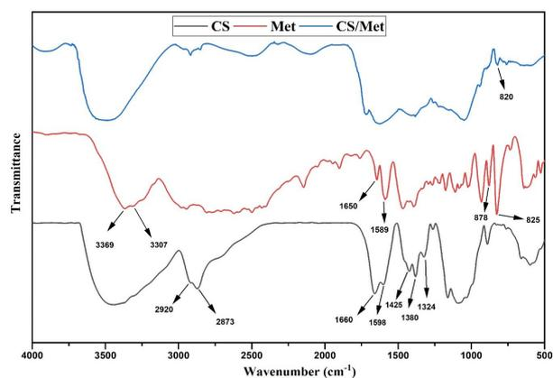
**Figure 1.** FTIR Spectrum of Chitosan Hydrogel (CS), Metformin Drug (Met) and Metformin Drug Loaded in Chitosan Hydrogel (CS/Met)
