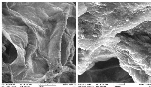
Figure 2. Scanning Electron Microscopy Micrograph CH/Met Hydrogel.
